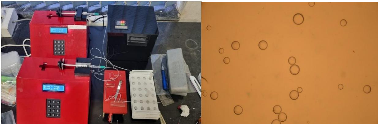
The microfluidic droplet setup as shown above comprises of two (2) syringe pumps, a glass droplet microfluidic device with two (2) inputs and one (1) output, a heating bed to heat the microfluidic device to a set temperature, a temperature controller, and a temperature feedback sensor.
