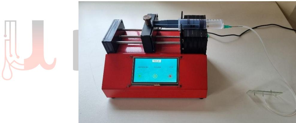
The Syringe Pump developed by us is a near-pulseless pump having a capacity to pump fluid at flow rates as low as  $1\mu\text{L}/\text{min}$  to as high as  $2000\mu\text{L}/\text{min}$ . The pump can handle syringes of 1mL, 2mL, 5mL, 10mL, and 20mL capacities, and it features an intuitive touchscreen as an HMI to get user input.
